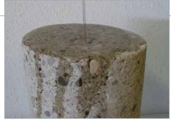
Without the drainable polymer additive water remains on the surface and can cause dangerous aquaplaning.
