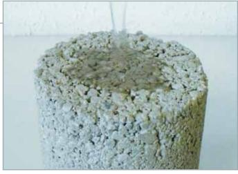
By using Nanoalps® System DRAIN the water seeps into the lower layers and allows for a dry surface.
